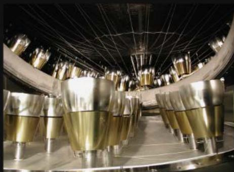
Internal view of the Borexino liquid scintillator containment vessel. From the photo several parts of the detector are visible: the photomultipliers (silver-like color) the mu-metal shielding (brass-like color) the bottom of the outer nylon vessel (upper part of the photo).
